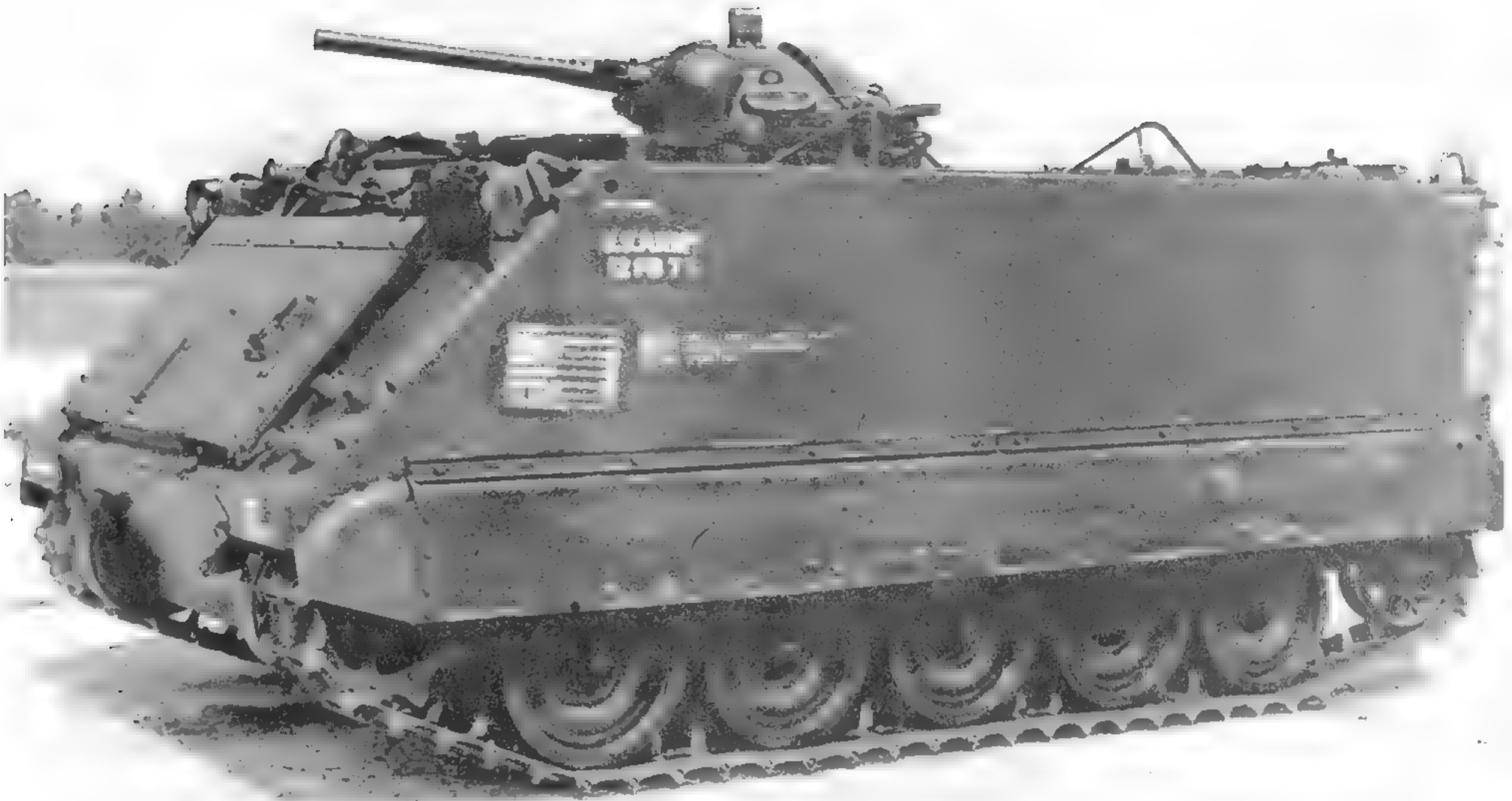
The M132A1 self-propelled flame thrower was one of the most fearsome weapons ever mounted on the M113 platform. Not visible is the 7.62 coaxial mounted machine gun. (U.S. Army photo)
